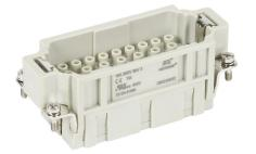
METE male insert, connector housing size 16B, 32-pole, crimped contact, 16 amp, 600 VAC/VDC, poles numbered 1 to 32. For use with METE multi-wire housings. Requires 16 amp male contacts METE 14106xxx.
