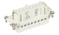
METE female insert, connector housing size 16B, 16-pole, screw terminals, accepts wire size 18-14 AWG, 16 amp, 600 VAC/VDC, poles numbered 1 to 16. For use with METE multi-wire housings.
