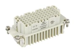
METE female insert, connector housing size 16B, 72-pole, crimped contact, 10 amp, 600 VAC/VDC, poles numbered 1 to 72. For use with METE multi-wire housings. Requires 10 amp female contacts METE 14103xxx.
