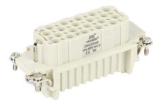
METE female insert, connector housing size 16B, 40-pole, crimped contact, 10 amp, 600 VAC/VDC, poles numbered 1 to 40. For use with METE multi-wire housings. Requires 10 amp female contacts METE 14103xxx.
