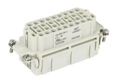
METE female insert, connector housing size 16B, 32-pole, crimped contact, 16 amp, 600 VAC/VDC, poles numbered 1 to 32. For use with METE multi-wire housings. Requires 16 amp female contacts METE 14105xxx.
