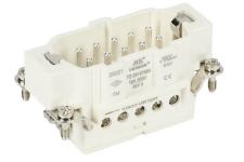
METE male insert, connector housing size 10B, 10-pole, screw terminals, accepts wire size 18-14 AWG, 16 amp, 600 VAC/VDC, poles numbered 1 to 10. For use with METE multi-wire housings.
