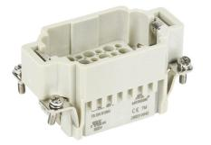
METE male insert, connector housing size 10B, 42-pole, crimped contact, 10 amp, 600 VAC/VDC, poles numbered 1 to 42. For use with METE multi-wire housings. Requires 10 amp male contacts METE 14104xxx.
