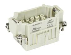
METE male insert, connector housing size 10B, 18-pole, crimped contact, 16 amp, 600 VAC/VDC, poles numbered 1 to 18. For use with METE multi-wire housings. Requires 16 amp male contacts METE 14106xxx.
