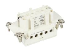
METE female insert, connector housing size 10B, 10-pole, screw terminals, accepts wire size 18-14 AWG, 16 amp, 600 VAC/VDC, poles numbered 1 to 10. For use with METE multi-wire housings.
