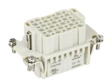
METE female insert, connector housing size 10B, 42-pole, crimped contact, 10 amp, 600 VAC/VDC, poles numbered 1 to 42. For use with METE multi-wire housings. Requires 10 amp female contacts METE 14103xxx.
