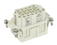
METE female insert, connector housing size 10B, 18-pole, crimped contact, 16 amp, 600 VAC/VDC, poles numbered 1 to 18. For use with METE multi-wire housings. Requires 16 amp female contacts METE 14105xxx.
