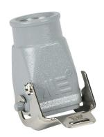
METE coupler housing, single lever, top entry, connector housing size 3A, (1) 3/8 NPT threaded hole, heavy-duty die cast aluminum. For use with METE size 3A 2-peg connector housings with male inserts.
