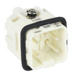
METE male insert, connector housing size 3A, 4-pole, screw terminals, accepts wire size 18-14 AWG, 10 amp, 600 VAC/VDC, poles numbered 1 to 4. For use with METE multi-wire housings.
