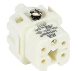
METE female insert, connector housing size 3A, 4-pole, screw terminals, accepts wire size 18-14 AWG, 10 amp, 600 VAC/VDC, poles numbered 1 to 4. For use with METE multi-wire housings.
