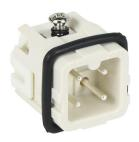
METE male insert, connector housing size 3A, 3-pole, screw terminals, accepts wire size 18-14 AWG, 10 amp, 600 VAC/VDC, poles numbered 1 to 3. For use with METE multi-wire housings.
