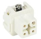
METE female insert, connector housing size 3A, 3-pole, screw terminals, accepts wire size 8-14 AWG, 10 amp, 600 VAC/VDC, poles numbered 1 to 3. For use with METE multi-wire housings.
