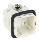
METE male insert, connector housing size 3A, 2-pole, screw terminals, accepts wire size 8-14 AWG, 10 amp, 600 VAC/VDC, poles numbered 2 to 3. For use with METE multi-wire housings.
