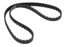
SureMotion timing belt, 3/8in L pitch, 1/2in wide, 76 tooth, 28.5in pitch length (circumference), neoprene, fiberglass reinforced.
