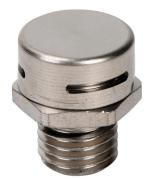
Stego pressure relief vent plug, M12 x 1.5mm thread type, nickel plated aluminum, 3,667 mL/min @ 70 mBar (1 psi), IP66 IP67.
