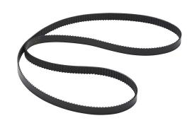
SureMotion timing belt, 0.08in MXL pitch, 1/4in wide, 280 tooth, 22.4in pitch length (circumference), polyurethane, polyester reinforced. Package of 3.
