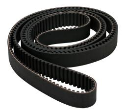
SureMotion timing belt, 8mm 8M pitch, 30mm wide, 350 tooth, 2800mm pitch length (circumference), neoprene, fiberglass reinforced.
