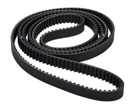
SureMotion timing belt, 8mm 8M pitch, 20mm wide, 350 tooth, 2800mm pitch length (circumference), neoprene, fiberglass reinforced.
