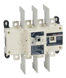
Socomec SIRCO DC series rotary disconnect switch, load break capable, 4-pole, 1000 VDC, 250A, 10kA SCCR, panel mount, UL 98B rated, front operated, accepts 10 x 10mm size shaft.
