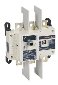
Socomec SIRCO DC series rotary disconnect switch, load break capable, 3-pole, 600 VDC, 250A, 10kA SCCR, panel mount, UL 98B rated, front operated, accepts  $10 \times 10 \text{mm}$  size shaft.
