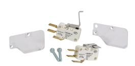
Socomec auxiliary contact, front mount, (1) N.O./(1) N.C. contact(s), 1A @ 125 VAC, low impedance. Package of 2. For use with SIRCO 100 - 600A switch bodies.
