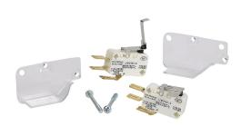
Socomec auxiliary contact, front mount, (1) N.O./(1) N.C. contact(s), 10A @ 125 VAC. Package of 2. For use with SIRCO 100 - 600A switch bodies.
