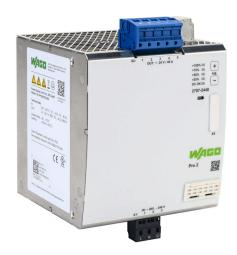
WAGO Pro2 series switching power supply, 24 VDC @ 40A/960W (adjustable), 220 VAC nominal input, 1-phase, enclosed, metal housing, 35mm DIN rail mount, cage clamp.
