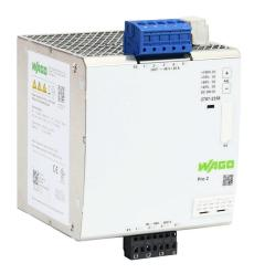
WAGO Pro2 series switching power supply, 48 VDC @ 20A/960W (adjustable), 480 VAC nominal input, 3-phase, enclosed, metal housing, 35mm DIN rail mount, cage clamp.
