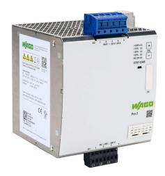
WAGO Pro2 series switching power supply, 24 VDC @ 40A/960W (adjustable), 480 VAC nominal input, 3-phase, enclosed, metal housing, 35mm DIN rail mount, cage clamp.
