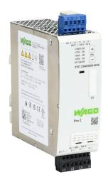
WAGO Pro2 series switching power supply, 24 VDC @ 10A/240W (adjustable), 480 VAC nominal input, 3-phase, enclosed, metal housing, 35mm DIN rail mount, cage clamp.
