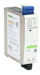
WAGO Pro2 series switching power supply, 24 VDC @ 5A/120W (adjustable), 480 VAC nominal input, 3-phase, enclosed, metal housing, 35mm DIN rail mount, cage clamp.
