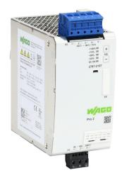
WAGO Pro2 series switching power supply, 48 VDC @ 10A/480W (adjustable), 120/240 VAC nominal input, 1-phase, enclosed, metal housing, 35mm DIN rail mount, cage clamp.
