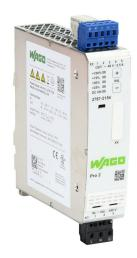
WAGO Pro2 series switching power supply, 48 VDC @ 2.5A/120W (adjustable), 120/240 VAC nominal input, 1-phase, enclosed, metal housing, 35mm DIN rail mount, cage clamp.
