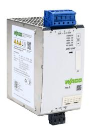
WAGO Pro2 series switching power supply, 24 VDC @ 20A/480W (adjustable), 120/240 VAC nominal input, 1-phase, enclosed, metal housing, 35mm DIN rail mount, cage clamp.
