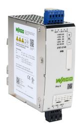
WAGO Pro2 series switching power supply, 24 VDC @ 10A/240W (adjustable), 120/240 VAC nominal input, 1-phase, enclosed, metal housing, 35mm DIN rail mount, cage clamp.
