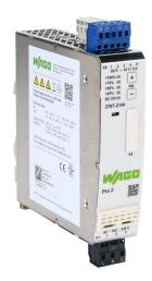
WAGO Pro2 series switching power supply, 24 VDC @ 5A/120W (adjustable), 120/240 VAC nominal input, 1-phase, enclosed, metal housing, 35mm DIN rail mount, cage clamp.
