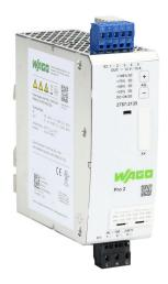
WAGO Pro2 series switching power supply, 12 VDC @ 15A/180W (adjustable), 120/240 VAC nominal input, 1-phase, enclosed, metal housing, 35mm DIN rail mount, cage clamp.
