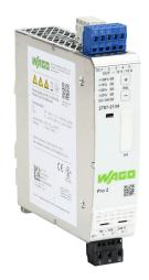
WAGO Pro2 series switching power supply, 12 VDC @ 10A/120W (adjustable), 120/240 VAC nominal input, 1-phase, enclosed, metal housing, 35mm DIN rail mount, cage clamp.
