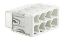
WAGO 2773 series splicing connector, push-in, side-entry, 8 openings, copper conductor, 20-12 AWG solid, 18-12 AWG stranded, 20A, 600V, polycarbonate housing, transparent/light gray. Package of 40.
