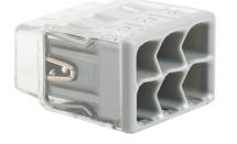
WAGO 2773 series splicing connector, push-in, side-entry, 6 openings, copper conductor, 20-12 AWG solid, 18-12 AWG stranded, 20A, 600V, polycarbonate housing, transparent/gray. Package of 50.
