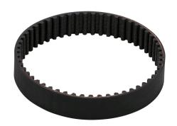
SureMotion timing belt, 5mm 5M pitch, 15mm wide, 55 tooth, 275mm pitch length (circumference), neoprene, fiberglass reinforced.
