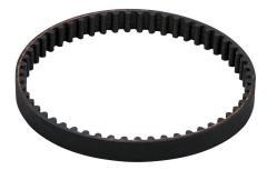
SureMotion timing belt, 5mm 5M pitch, 9mm wide, 55 tooth, 275mm pitch length (circumference), neoprene, fiberglass reinforced.
