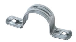
Minerallac 2-hole conduit mount strap, standard duty, UL Type UL 1565. Package of 100. For use with 1-1/4in RMC/IMC/LFMC, 1-1/2in EMT, 1-1/2in FMC.
