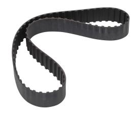
SureMotion timing belt, 3/8in L pitch, 1in wide, 72 tooth, 27in pitch length (circumference), neoprene, fiberglass reinforced.
