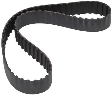
SureMotion timing belt, 3/8in L pitch, 1in wide, 72 tooth, 27in pitch length (circumference), neoprene, fiberglass reinforced.
