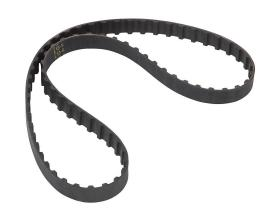
SureMotion timing belt, 3/8in L pitch, 1/2in wide, 72 tooth, 27in pitch length (circumference), neoprene, fiberglass reinforced.
