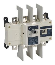
Socomec SIRCO series rotary disconnect switch, load break capable, 4-pole, 600 VAC, 200A, 200kA SCCR, panel mount, UL 98 rated, front operated, accepts 10 x 10mm size shaft.
