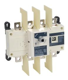
Socomec SIRCO series rotary disconnect switch, load break capable, 4-pole, 600 VAC, 100A, 200kA SCCR, panel mount, UL 98 rated, front operated, accepts 10 x 10mm size shaft.
