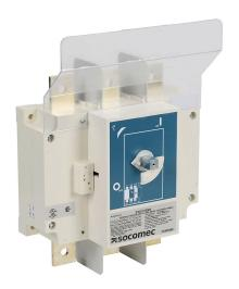
Socomec SIRCO series rotary disconnect switch, load break capable, 3-pole, 600 VAC, 600A, 200kA SCCR, panel mount, UL 98 rated, front operated, accepts 15 x 12mm size shaft.
