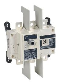
Socomec SIRCO series rotary disconnect switch, load break capable, 3-pole, 600 VAC, 200A, 200kA SCCR, panel mount, UL 98 rated, front operated, accepts 10 x 10mm size shaft.
