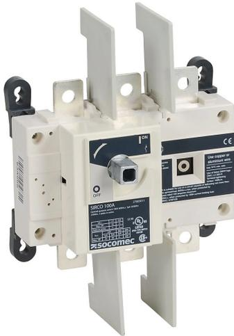
Socomec SIRCO series rotary disconnect switch, load break capable, 3-pole, 600 VAC, 100A, 200kA SCCR, panel mount, UL 98 rated, front operated, accepts 10 x 10mm size shaft.
